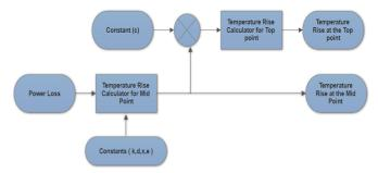
Figure 01 Temperature rise calculation as per IEC TR 60890[6]
